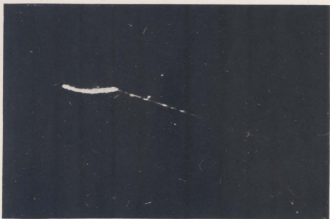
(c) The neutron here causes the transmutation of a nitrogen nucleus which it enters and by so doing occasions the ejection of an \alpha particle while the heavy, short trajectory reveals the recoil of the remainder of the nucleus. The pressure was here low and the magnification large.
